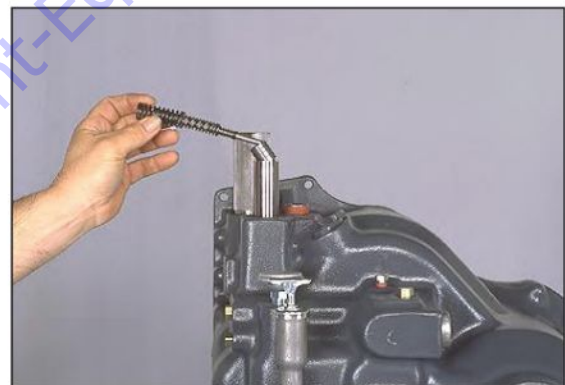
Figure 100 Remove Modulator Valve Components
