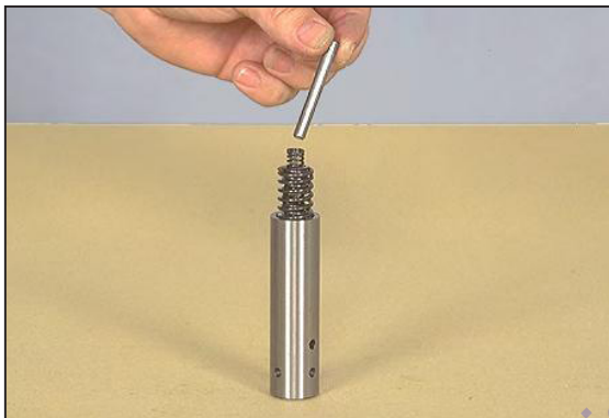
Figure 113 Install Stop Pin
