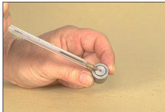
Figure 105 Verify Orifice is Clear of Debris
