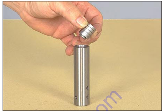
Figure 109 Position Accumulator Coil
