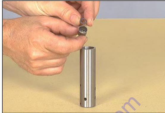
Figure 103 Install Spring Spacer
