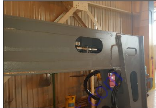
Figure 70 Boom Side Access Hole
