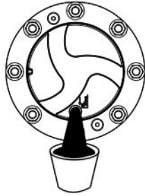
Figure 51 Draining Planetary Gear Oil
