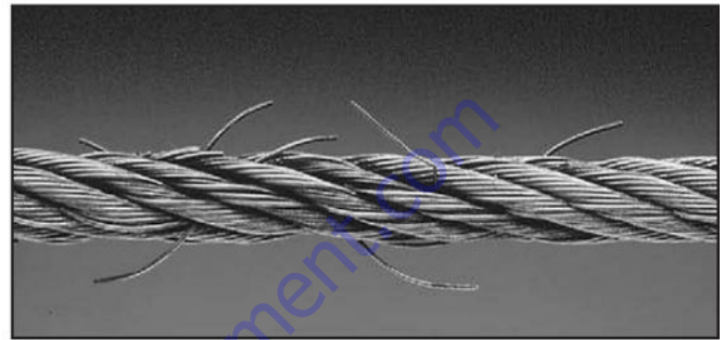
Cable with Broken Wires
