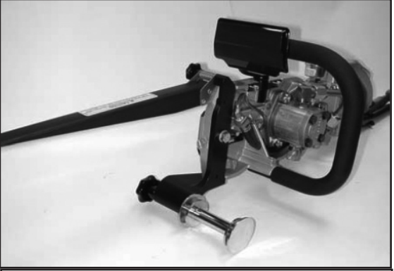
STEP 5 Insert axle into mounting bracket as shown and firmly tighten bolt
