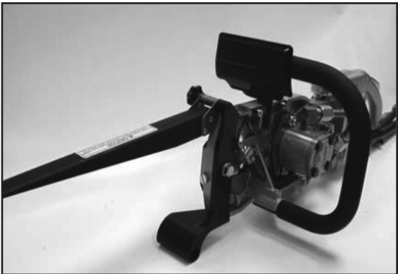
STEP 4 Attach SpeedHook® mounting bracket assy. Note: Do not over tighten attachment bolts
