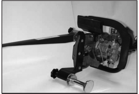
STEP 5 Insert axle into mounting bracket as shown and firmly tighten bolt
