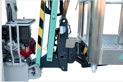
IM R 13 T compact jib assembly hosting both the load sensor and basket rotation system.
