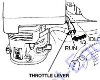
Figure 8. Throttle Lever (1/3 Start Position
