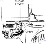
Figure 10. Engine Choke Lever (Open)
