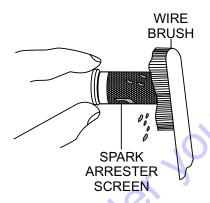
Figure 23. Cleaning The Spark Arrester
