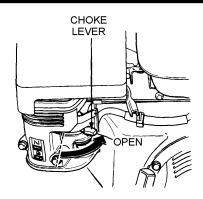
Figure 13. Choke Lever (Open)
