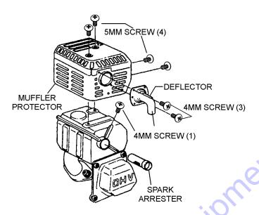
Figure 22. Spark Arrester Removal
