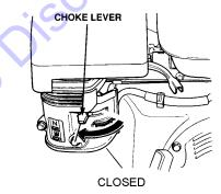
Figure 9. Engine Choke Lever (Closed)
