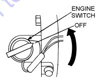
Figure 16. Engine ON/OFF Switch (OFF)
