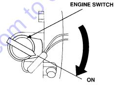
Figure 11. Engine ON/OFF Switch (ON Position)
