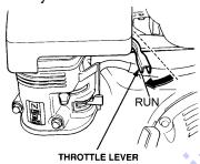
Figure 14. Throttle Lever (Run)
