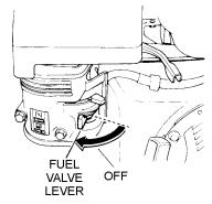
Figure 17. Fuel Valve Lever (OFF)
