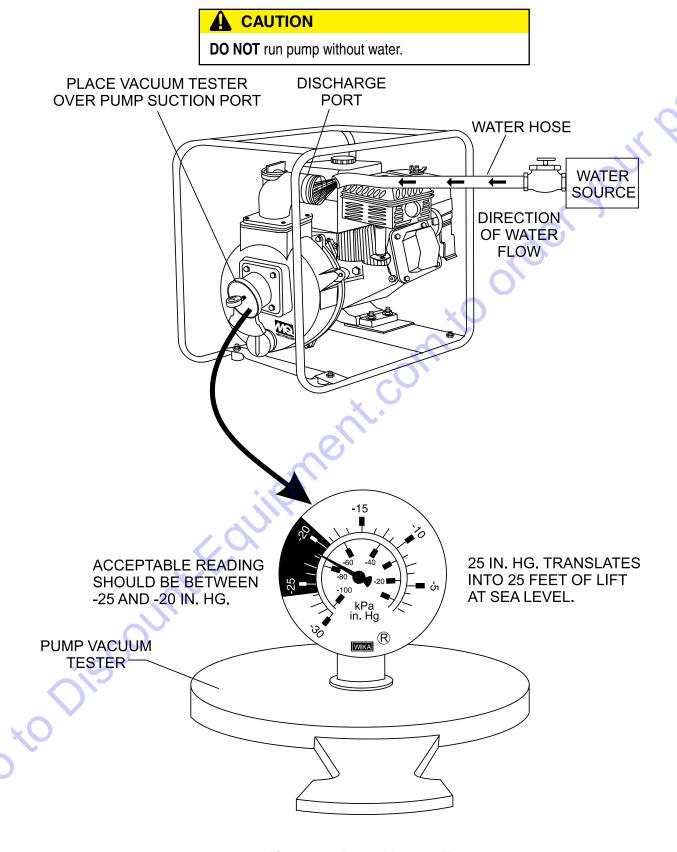
Figure 18. Pump Vacuum Tester
