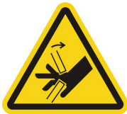
Pinch Point Hazard
