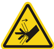
Pinch Point Hazard
