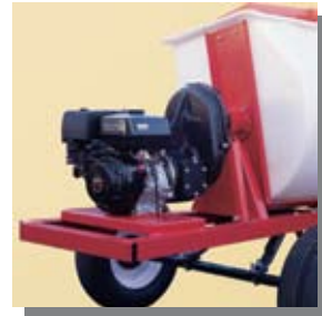
Totally enclosed transmission eliminates wear due to dust contamination.
