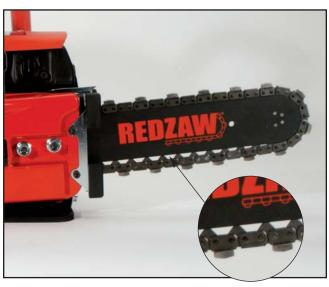
Proper Chain tensions can have a gap as loose as 3/4" between the bar and chain
