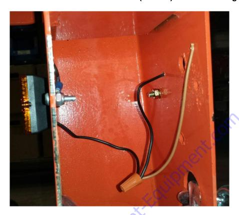
7) Connect the 4" wire (connecting front lights) to the light brown wire on the main light kit wire using the tap connector.
