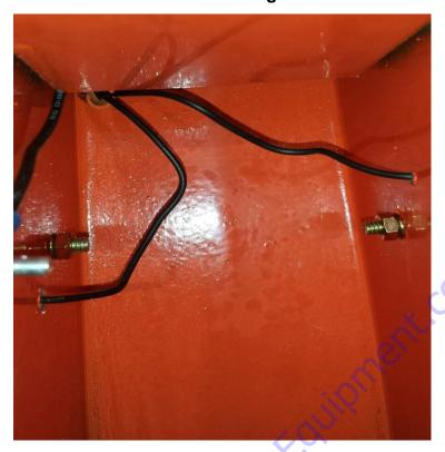
9) Install adhesive cable mounts & frame wire clips to hood area.
