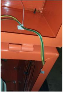
11) Tighten license plate holder and lights to inside of the hood. From the adhesive cable mount from top of the hood, there should be 4 feet of wire. Cut the extra off. Tie the extra 4 feet of wire remaining to the extra connection wire that came with light kit. Tape it to the license plate holder.
