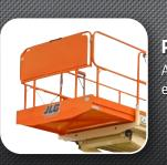
**Platform Extension** A standard feature, the platform extension has a 250 lb capacity.
