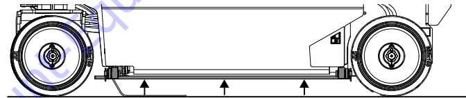
Platform Fully Lowered - Pothole Bars Raised
