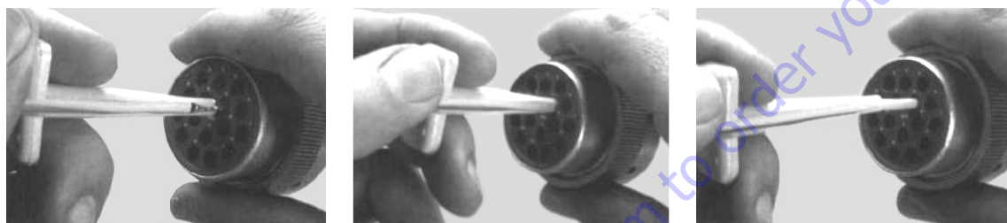
Figure 8-16. HD/HDP Contact Removal
