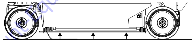
Platform Fully Lowered - Pothole Bars Raised
