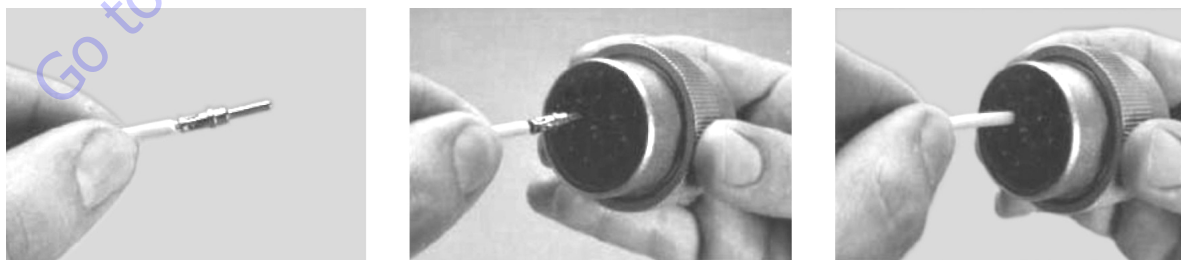
Figure 7-14. HD/HDP Contact Installation
