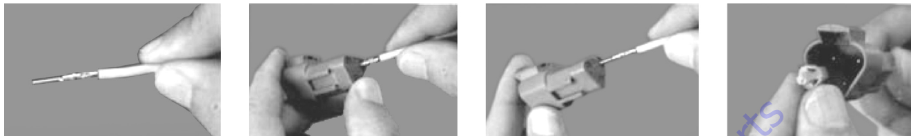
Figure 7-12. DT/DTP Contact Installation
