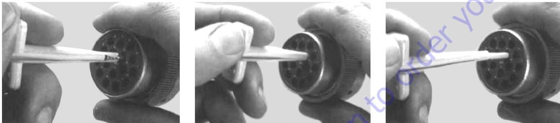
Figure 7-16. HD/HDP Contact Removal
