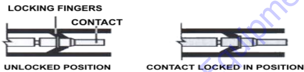
Figure 6-15. HD/HDP Locking Contacts into Position
