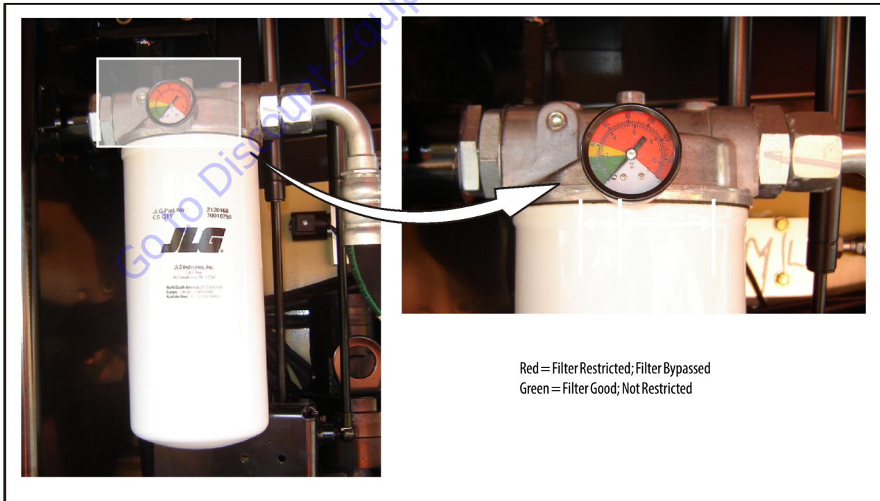
Figure 5-43. Hydraulic Return Filter Condition Indicator
