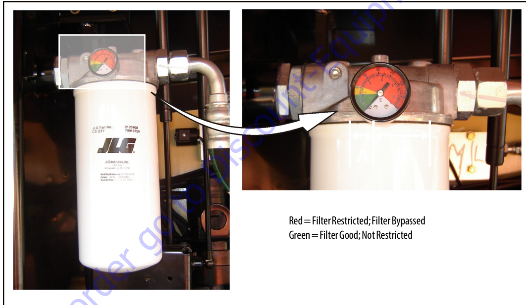
Figure 7-7. Hydraulic Return Filter Condition Indicator
