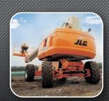
**Solid Ground** 45% gradeability and oscillating axle for improved traction.
