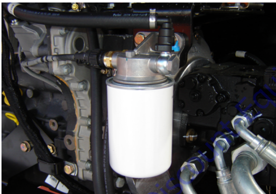
Figure 3-62. Location of the Fuel Filter
