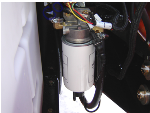
Figure 3-63. Location of the Fuel Pre-Filter
