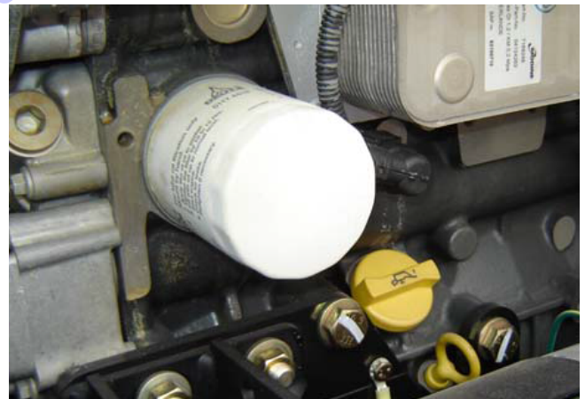
Figure 3-61. Location of the Oil Filter
