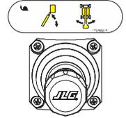
**NOTE:** Lower lift will not function when operating main lift.
