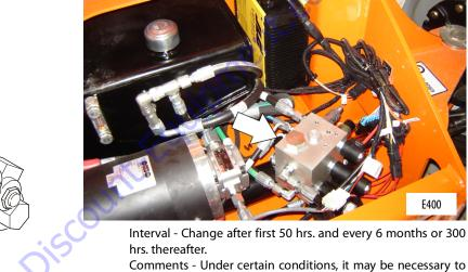
Comments - Under certain conditions, it may be necessary to replace the hydraulic filter on a more frequent basis. A common symptom of a dirty filter is sluggishness experienced in hydraulic functions.
