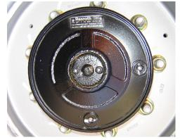
Lube Point(s) - Level/Fill Plug Capacity - 17 oz. (1/2 Full) Lube - EPGL Interval - Check level every 3 months or 150 hrs of operation; change every 2 years or 1200 hours of operation
