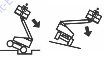
• Do not elevate platform or drive with platform elevated while on or near a sloping, uneven, or soft surface. Ensure machine is positioned on a smooth, firm surface within the limits of the maximum operating slope before elevating platform or driving with the platform in the elevated position.
