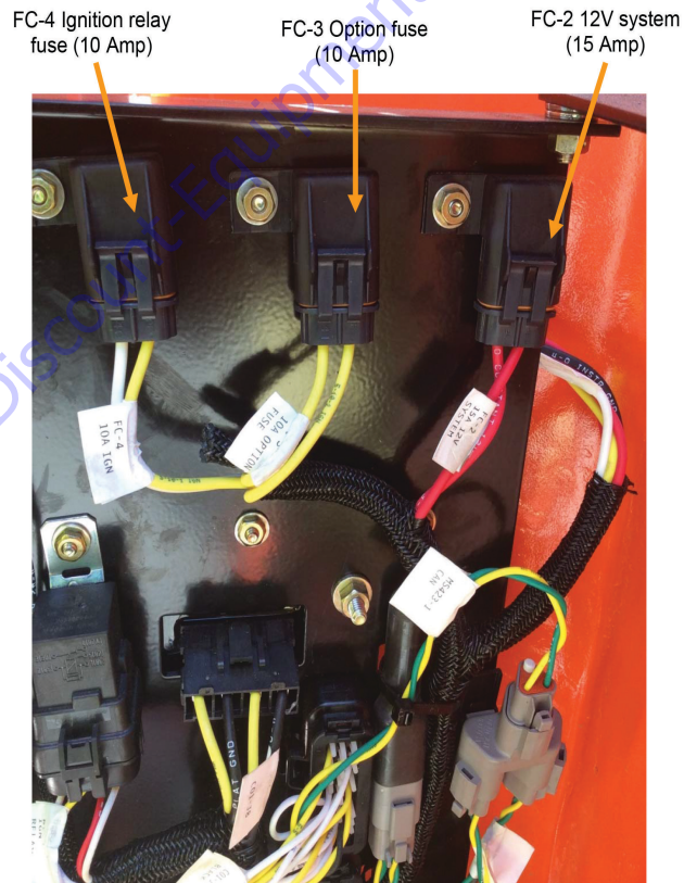
Figure 3-7. System Fuses
