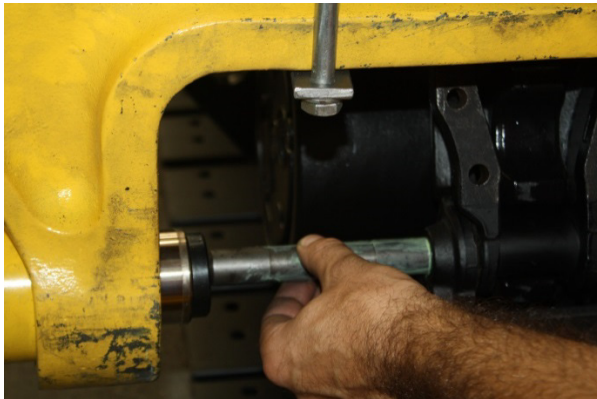
Figure 3-20. Installing Master Pin
