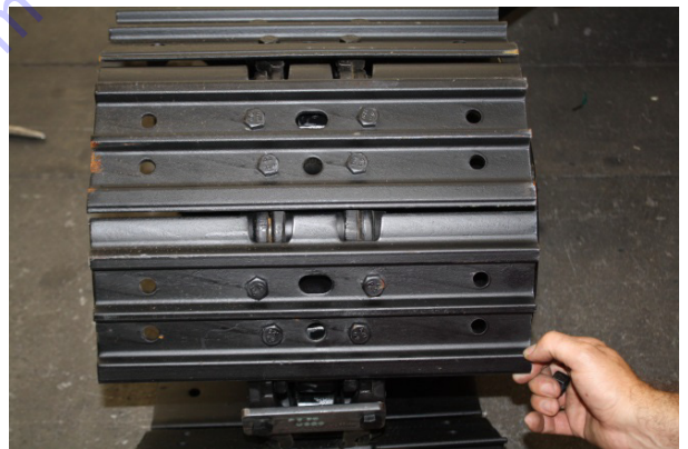
Figure 3-23. Reinstall Triple Grouser Shoes
