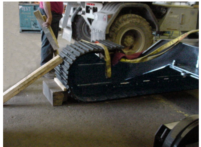
Figure 3-15. Brace Steel Track
