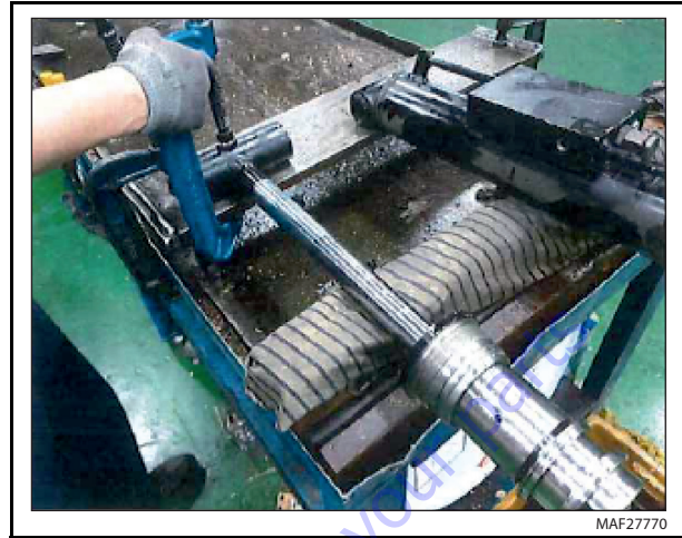
Figure 5-32. Cylinder Rod Support
