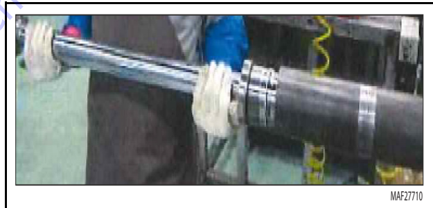
Figure 5-33. Cylinder Rod Installation
