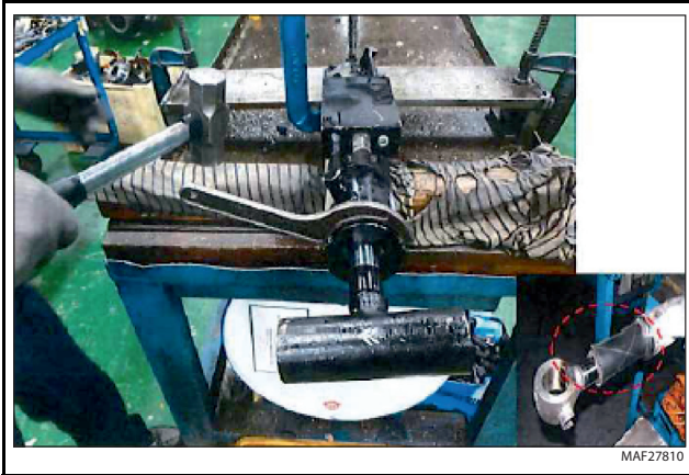
Figure 5-18. Cylinder Head Cover Removal
