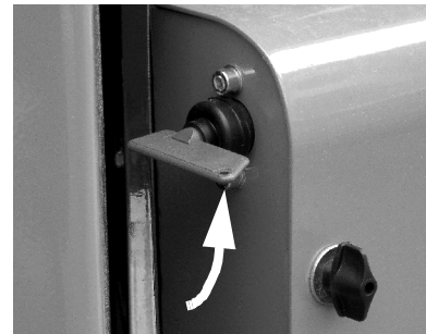
BATTERY DISCONNECT - GAS/AC-ELECTRIC
