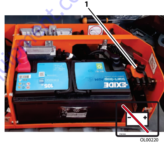
BATTERY DISCONNECT SWITCH - DIESEL/AC-ELECTRIC
