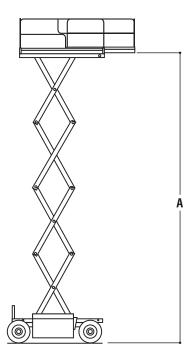
A. Platform Height Elevated 26 ft (7.9 m) B. Platform Height Lowered 4 ft 1.5 in. (1.3 m) C. Platform Railing Height 3 ft 7.5 in. (1.1 m) D. Overall Height 7 ft 9.5 in. (2.4 m) E. Platform Size 65 x 102 in. (1.65 x 2.6 m) 4 ft (1.2 m) F. Platform Extension
