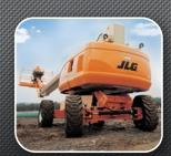
**Solid Ground** 45% gradeability and oscillating axle for improved traction.
