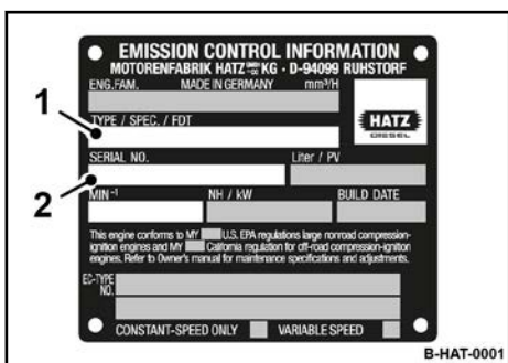
Fig. 2: Engine type plate (example)
