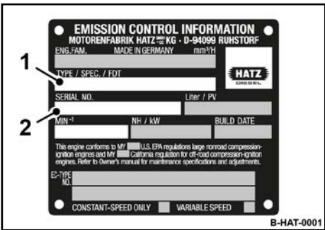
Fig. 2: Engine type plate (example)
