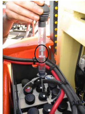
Figure 8-4. Measuring Electrolyte Specific Gravity
