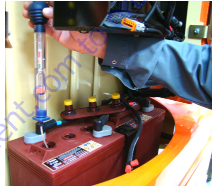
Figure 5-8. Measuring Electrolyte Specific Gravity
