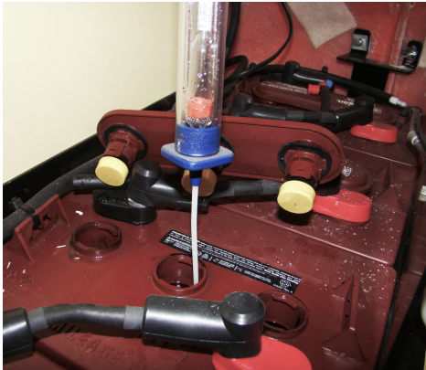
Figure 6-8. Measuring Electrolyte Specific Gravity
