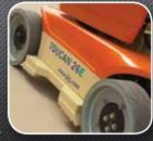
**Work Cleaner**Thick rubber non-marking tires leave facility floors intact.
