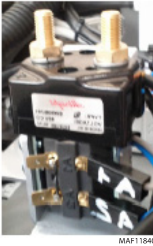
Figure 2-35. External Main Contactor
