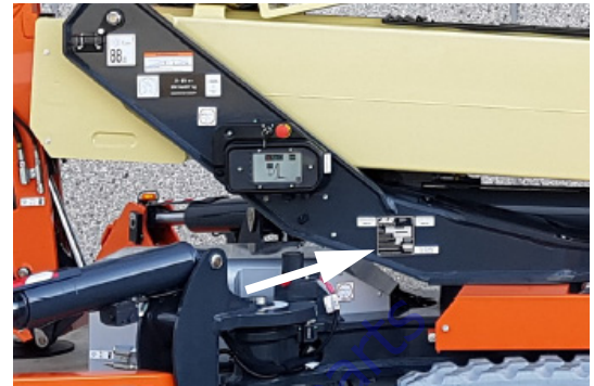
Figure 1-3. X33JP / X1000AJ Serial Number Plate Location (on side of turn table frame)
