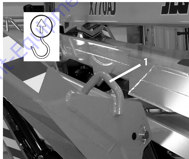
Figure 4-9. Machine Lifting Points
