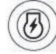
Figure 6-34. Allows the electric motor to be switched on/off. If the button is pressed with the engine on, this will be stopped.
