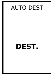
Figure 5-7. Outriggers Auto-Retraction In Progress
