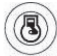
Figure 6-33. Allows the engine to be switched on/off. If the button is pressed with the engine on, this will be stopped.
