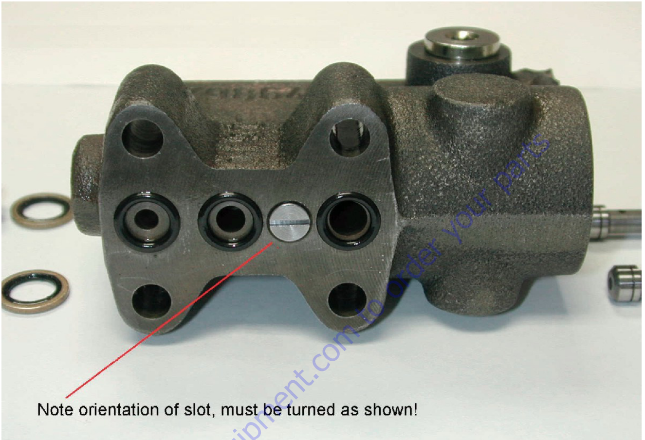
Figure 5-64. Function Pump, Pressure and Flow Control - Sheet 3
