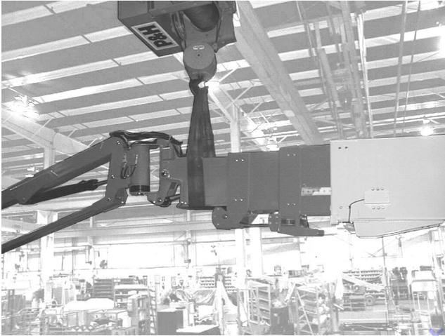
3. Place blocking under lift cylinder to hold it in place.
