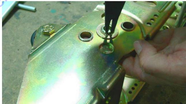
9. Remove the snap ring from the other side of the bracket.
