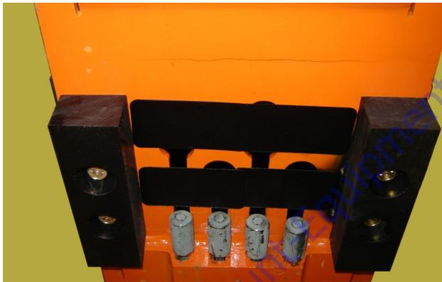
2. Fabricate a special fixture as shown below to keep four extend wire ropes from crossing over each other.
