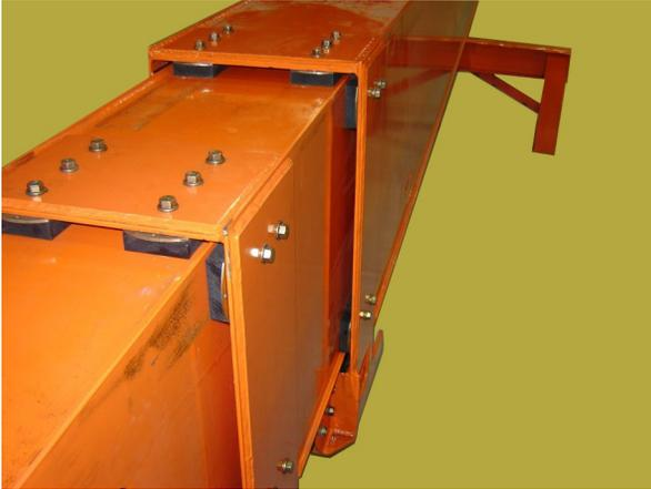
26. Put moly paste on the sheave mounts at the rear of the inner mid boom section and install the sheaves.
