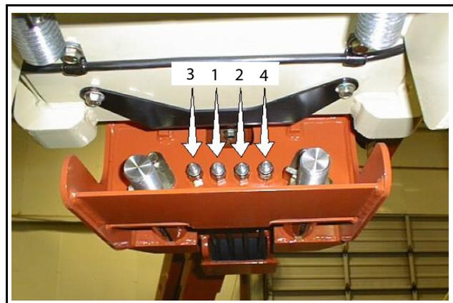
Figure 4-34. Torque Sequence for Fly Extend Rope
