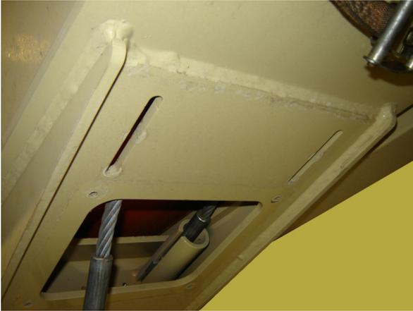
26. Remove the outer mid retract cables from the attachment fixtures at the front of the boom base section.
