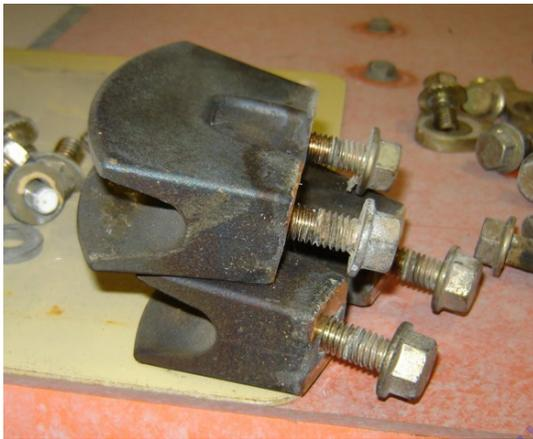
25. Remove the trunnion blocks that secure the telescope cylinder rod to the boom base section.
