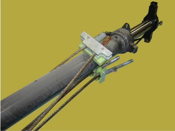
32. Remove the cable retainer plate, cable retainer block, bushing, and sheave.
