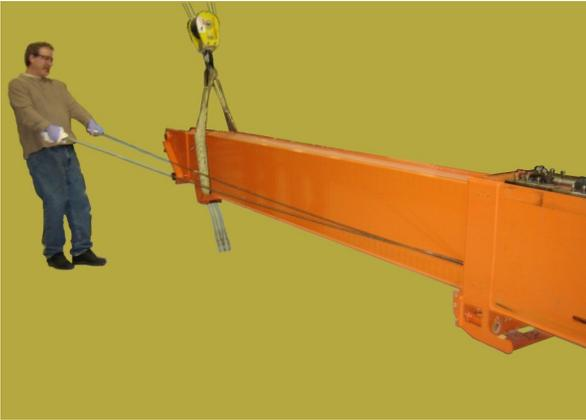
40. Remove the outer mid retract cables from the rear of the inner mid boom section.
