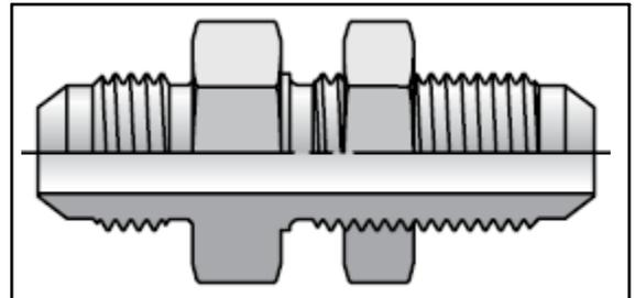
Figure 5-7. Bulkhead Thread
