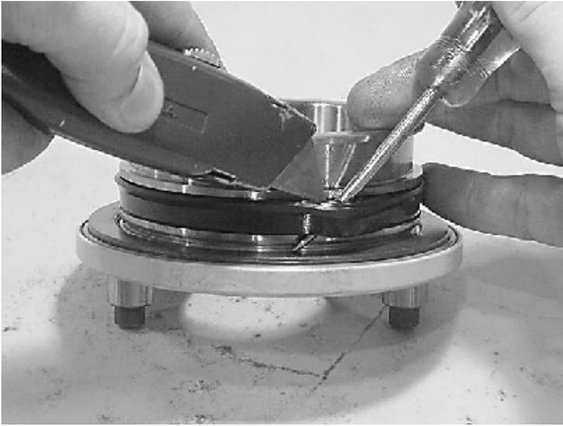
17. Remove the thrust washers (304), from the end cap (4) and shaft (2).
