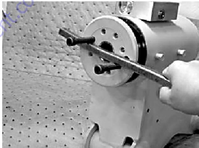
13. Install the stop tube onto the shaft end. Stop tube is an available option to limit the rotation of an actuator.
