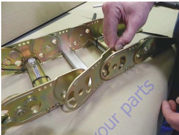
5. Remove the snap rings and pins.
