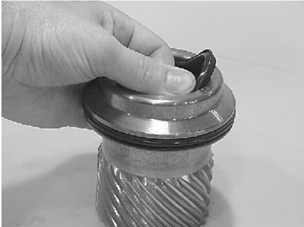
Beginning with the inner seal (200) insert one end of b/u ring in the lower groove and feed the rest in using a circular motion. Make sure the wedged ends overlap correctly.
