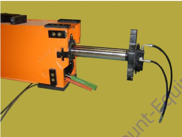
36. Install the cylinder trunnion blocks and shims.
