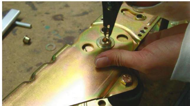
10. Push down with slight pressure on the link and slide the bracket side up and over the extrusion on the link.
