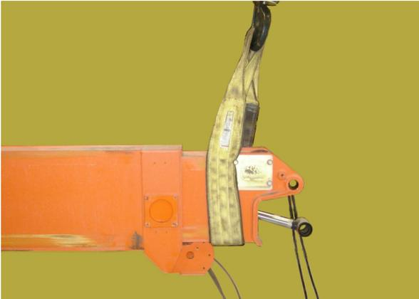
47. Remove the tape from the fly boom section and remove the fly boom retract cables.
