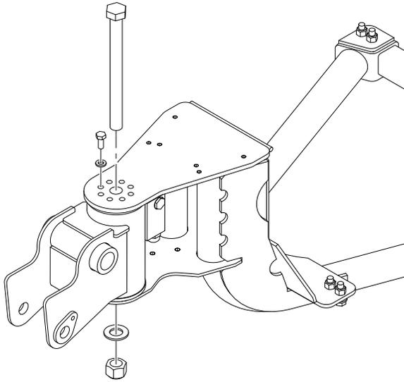
3. Apply JLG Threadlocker PN 0100011 to the eight bolts securing the support to the rotator and install the bolts.
