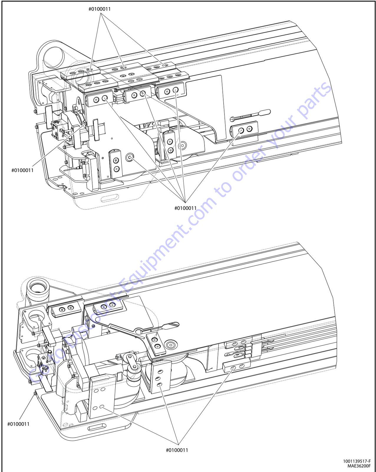
Figure 4-11. Locations for Threadlocker Application - Sheet 2 of 4
