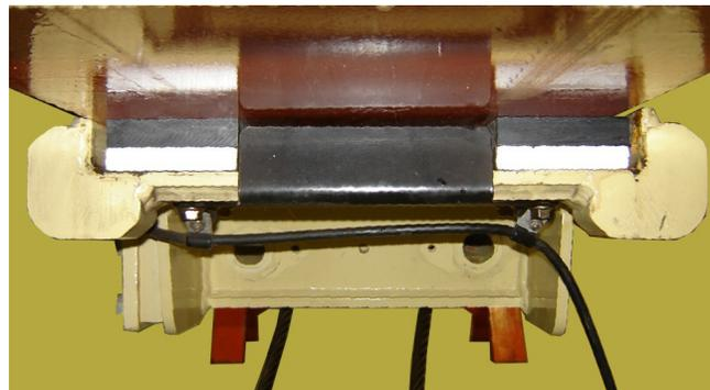
40. Push the inner mid boom assembly the rest of the way into the boom base section, adjusting the lifting device as necessary to keep the weight balanced.
