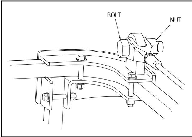
3. Install the Attachment Ring onto the cable.
