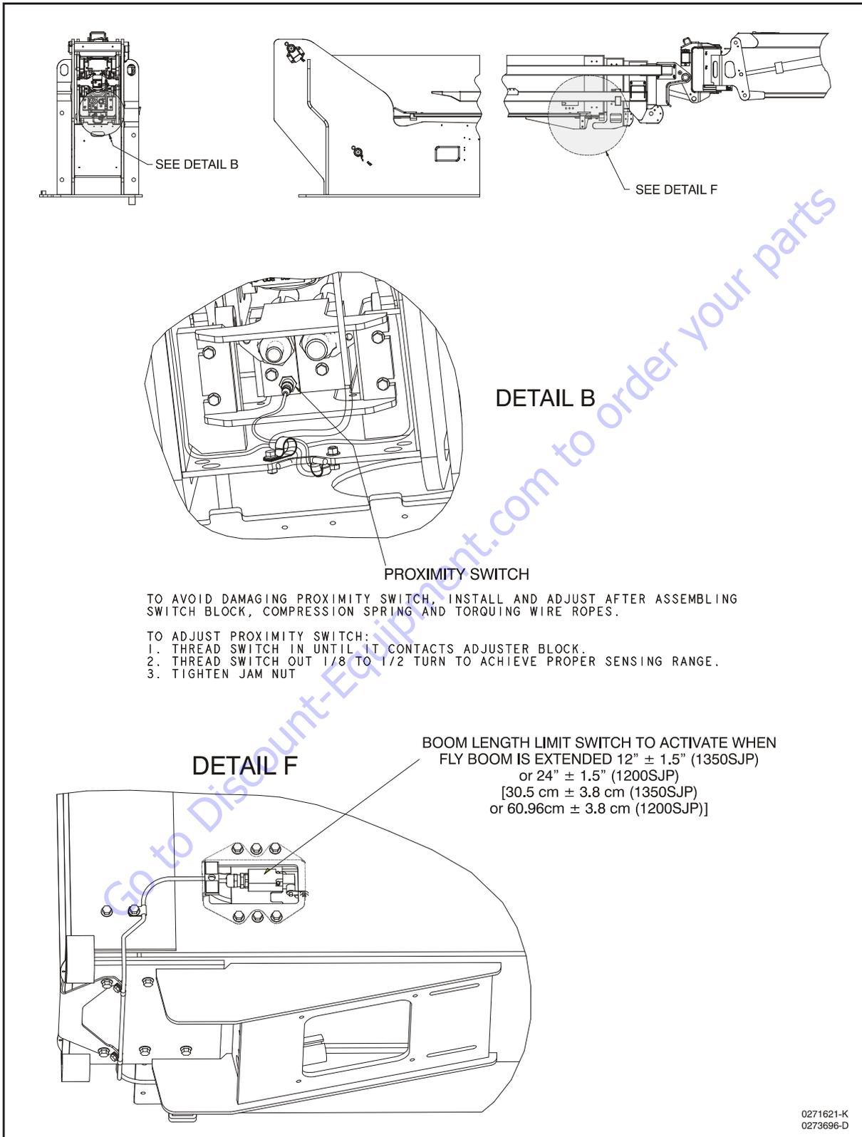
Figure 4-21. Boom/Jib Sensors and Switches Installation - Sheet 4 of 4
