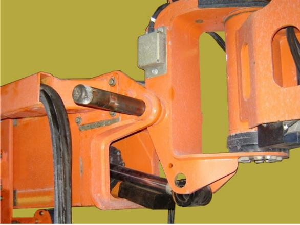
7. Remove the jib and platform assembly from the boom.
