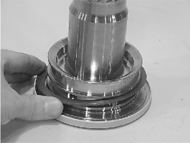
3. Install the wiper seal (304.1/green O-ring) into its groove on the shaft (2) and end cap (4) around the outside edge of the thrust washer (304).
