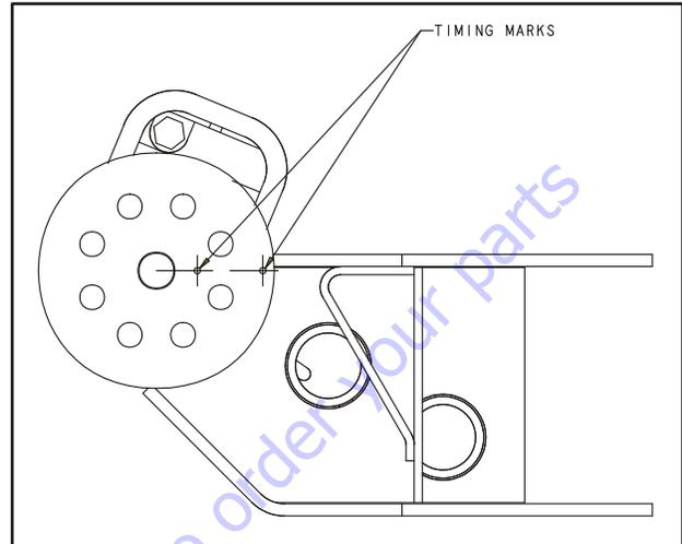
**Figure 4-16. Jib Rotator Orientation**
