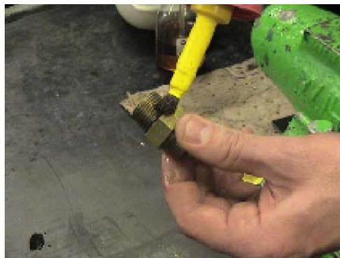
**5.2 HYDRAULIC CONNECTION ASSEMBLY AND TORQUE SPECIFICATION**
