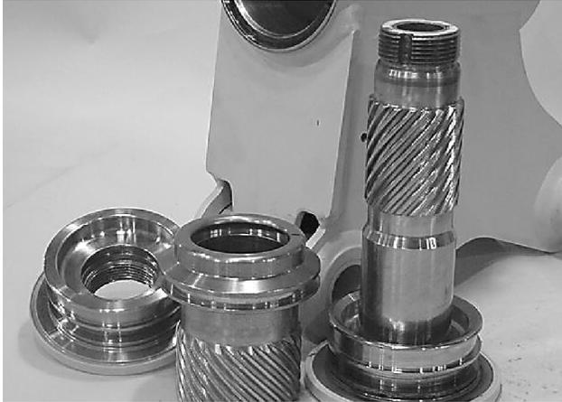
2. Inspect the thrust washers (304) for rough or worn edges and surfaces. Measure its thickness to make sure it is within specifications (Not less than 0.092" or 2.34 mm).
