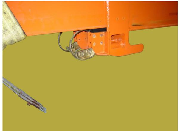
**NOTE:** When pulling the outer mid and fly boom sections out of the inner mid boom section, make sure the outer mid retract cables do not catch at the rear of the boom section.
