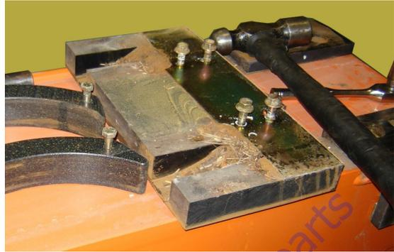
34. Remove the lock plates from the fly boom retract cable adjustment nuts and remove the adjustment nuts from the fly boom retract cables and from the fly boom extend cables at the front of the inner mid boom section.
