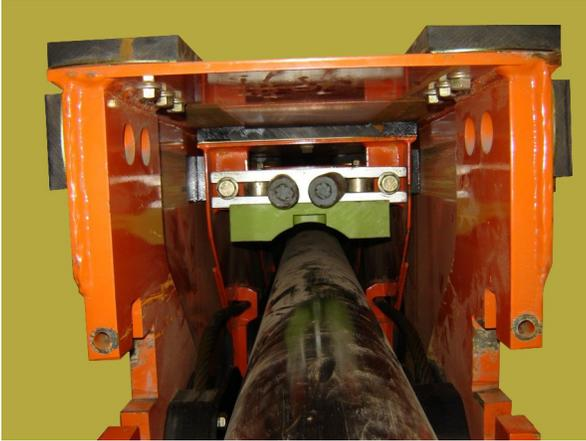
35. Push the cylinder the rest of the way into the inner mid boom assembly.
