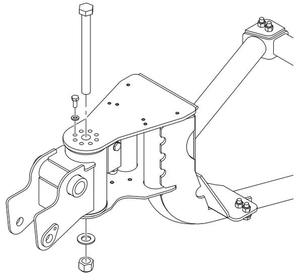
6. Remove the platform support from rotator.
