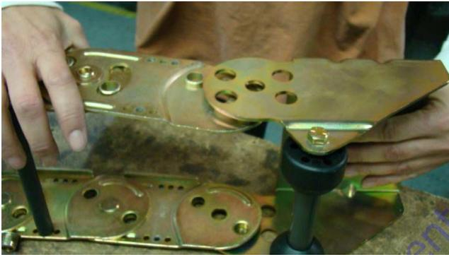
12. Slide the bracket off of the powertrack.
