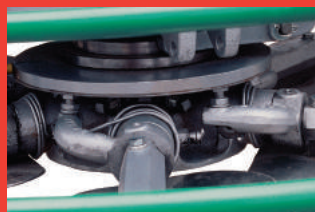
Spider assemblies feature long-lasting wear plates and spider hubs
