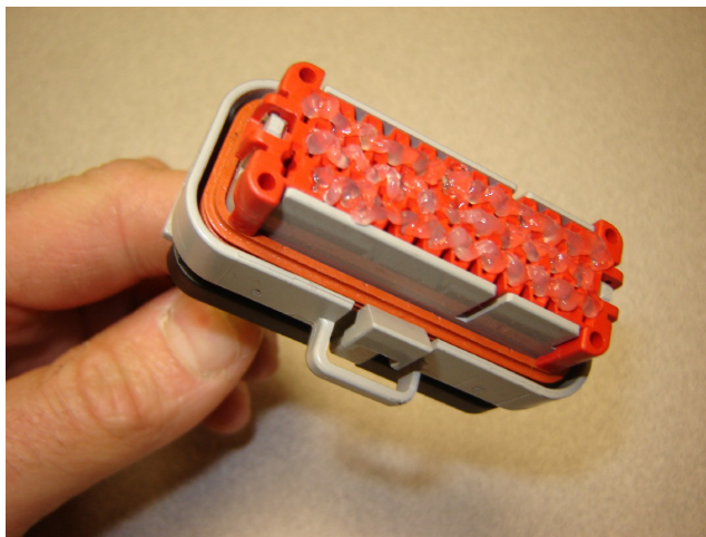
Figure 7-5. Application to plug/male connector housing
