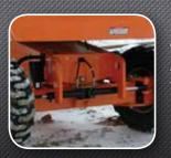
**45% Gradeability**An oscillating axle improves traction over mud and uneven terrain.
