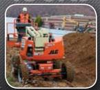
**45% Gradeability**Improved rough terrain capabilities for optimal off-slab productivity.
