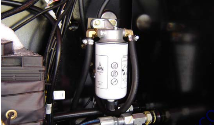
B. Fuel Filter - Deutz TD2.9 (On Hydraulic Tank)
