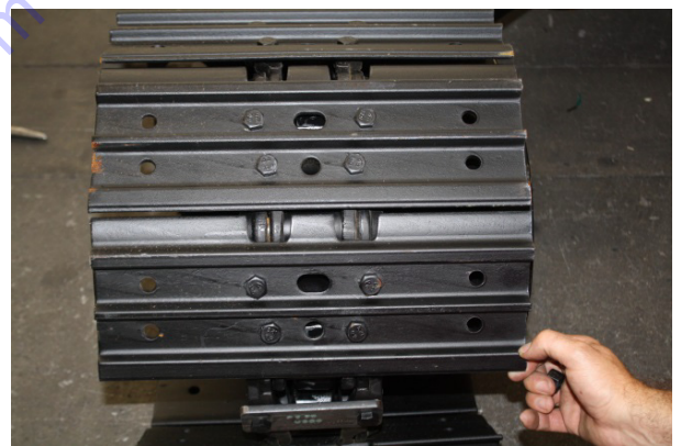
Figure 3-23. Reinstall Triple Grouser Shoes
