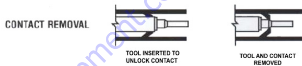
Figure 7-17. HD/HDP Unlocking Contacts
