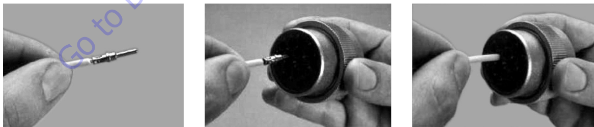
Figure 7-14. HD/HDP Contact Installation
