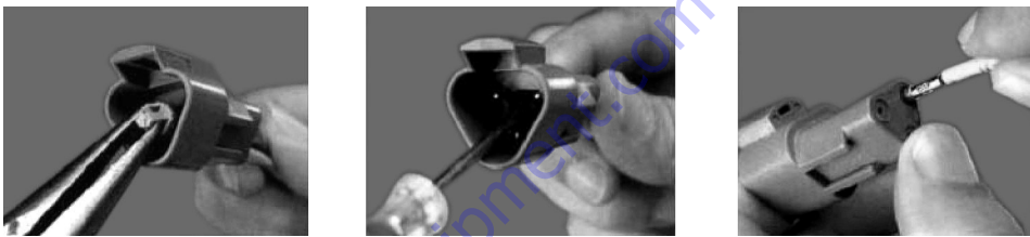
Figure 7-13. DT/DTP Contact Removal
