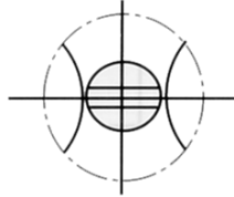
pressure compensator and flow control DFR One X - port is plugged.
