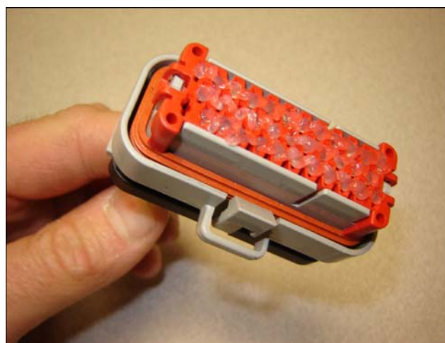
Figure 7-7. Application to plug/male connector housing
