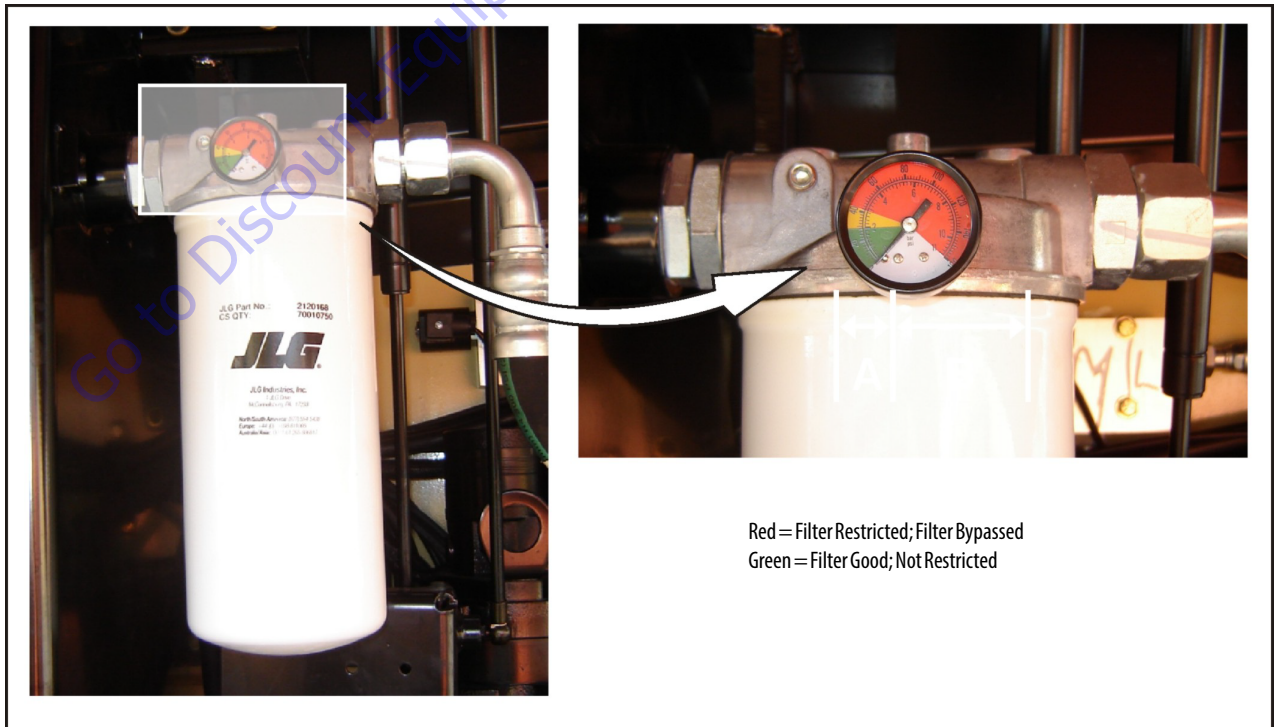
Figure 5-58. Hydraulic Return Filter Condition Indicator - SN 139396 to Present
